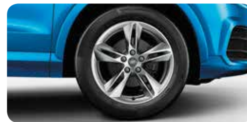
Cast aluminium wheels in 5-spoke dynamic design size 7 J x 18 with 235/50 R 18 tyres 1
