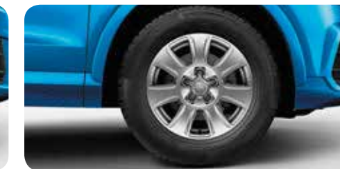
Forged aluminium winter wheels in 7-arm design size 6.5 J x 16 with 215/65 R 16 tyres 1 , can be fitted with snow chains, permissible top speed 210 km/h
