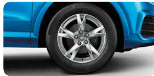
Cast aluminium wheels in 5-spoke Y design size 7 J x 17 with 235/55 R 17 tyres 1
