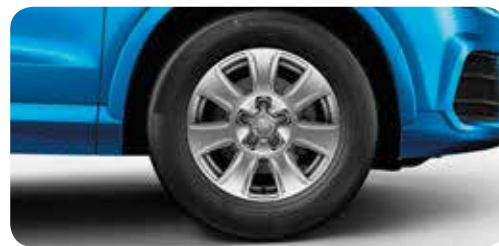
Forged aluminium wheels in 7-arm design size 6.5 J x 16 with 215/65 R 16 tyres 1
