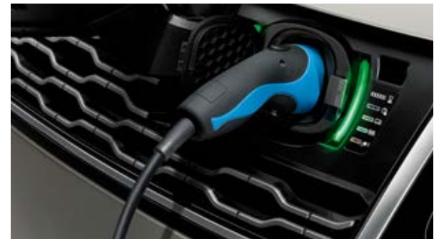
Public charging cable
