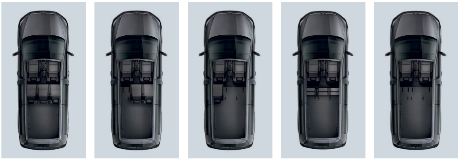
Standard five-seat layout. | 2nd row single seat removed. | 2nd row dual seat removed. | 2nd row seats folded. | 2nd row seats removed.
