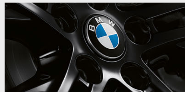
○ The floating hub cap consists of the BMW logo that no longer turns with the wheel but instead remains level. The hub cap can be mounted to all BMW light alloy wheels with a pitch circle diameter of 112 mm.
