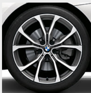
□ 19" light alloy wheels V-spoke style 772 in Bicolour Ferric Grey with mixed tyres, burnished, front wheel size 9J x 19, 255/35 ZR19 tyres, rear wheel size 10J x 19, 275/35 ZR19 tyres. 1,3
