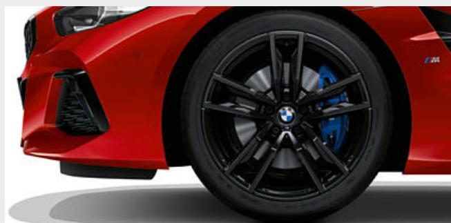
□ 19" M alloy wheels Double-spoke style 799 M in jet black uni with mixed tyres, front wheel size 9J x 19, 255/35 ZR19 tyres, rear wheel size 10J x 19, 275/35 ZR19 tyres. 4
