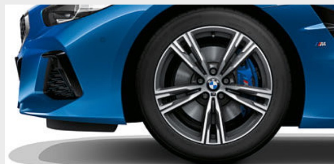
□ 18" M alloy wheels Double-spoke style 798 M in Bicolour Orbit Grey with mixed tyres, burnished, front wheel size 9J x 18, 255/40 ZR18 tyres, rear wheel size 10J x 18, 275/40 ZR18 tyres. 2,6
