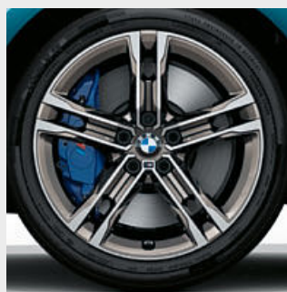
■ 18" M light alloy wheels Double-spoke style 556 M Bicolour Cerium Grey matt, gloss-lathed, wheel size 8J x 18 with 225/40 R18 tyres. 4
