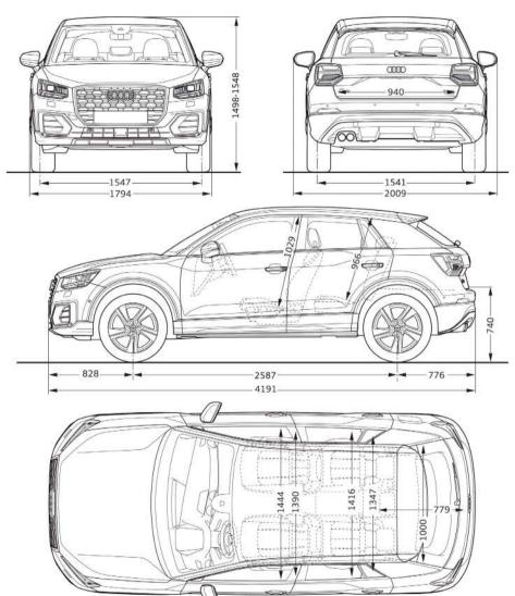
**Dimensions in millimetres.** Dimensions measured with vehicle at unladen weight. Luggage compartment volume: 405 / 1,050 l (measured by the VDA method using 200 x 100 x 50 mm blocks). Turning circle approx. 11.1 m.
