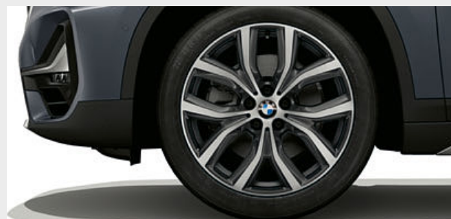
□ 19" light alloy wheels Y-spoke style 511 Orbit Grey with runflat tyres, gloss-lathed, 8J x 19 with 225/45 R19 tyres.
