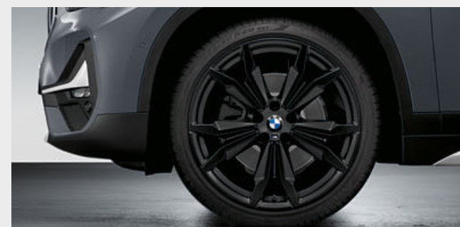
○ The high-quality 20" M light alloy wheels Double-spoke 717 M are designed in Jet Black matt, weight-optimised with flow forming and with M logo. TPMS summer complete wheel set with run-flat tyres, wheel size 8J x 20 with tyre size 225/40 R20 94Y RSC.
