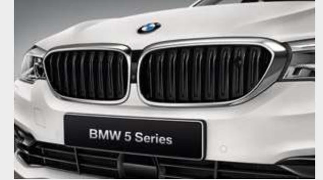
**Active Air Stream kidney grille** The air vents actively regulate the air stream. If the cooling demand for the engine increases, the air vents are opened.
