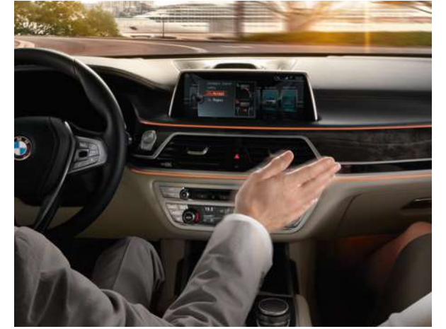
BMW Gesture Control allows for specified functions to be controlled with gestures.
