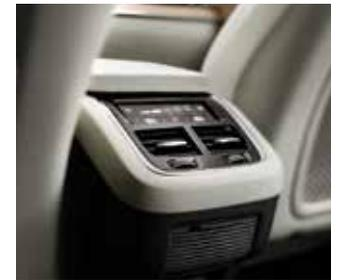
The 4 zone climate system can be controlled from the center touchscreen, or a graceful touch control panel at the end of the tunnel console.
