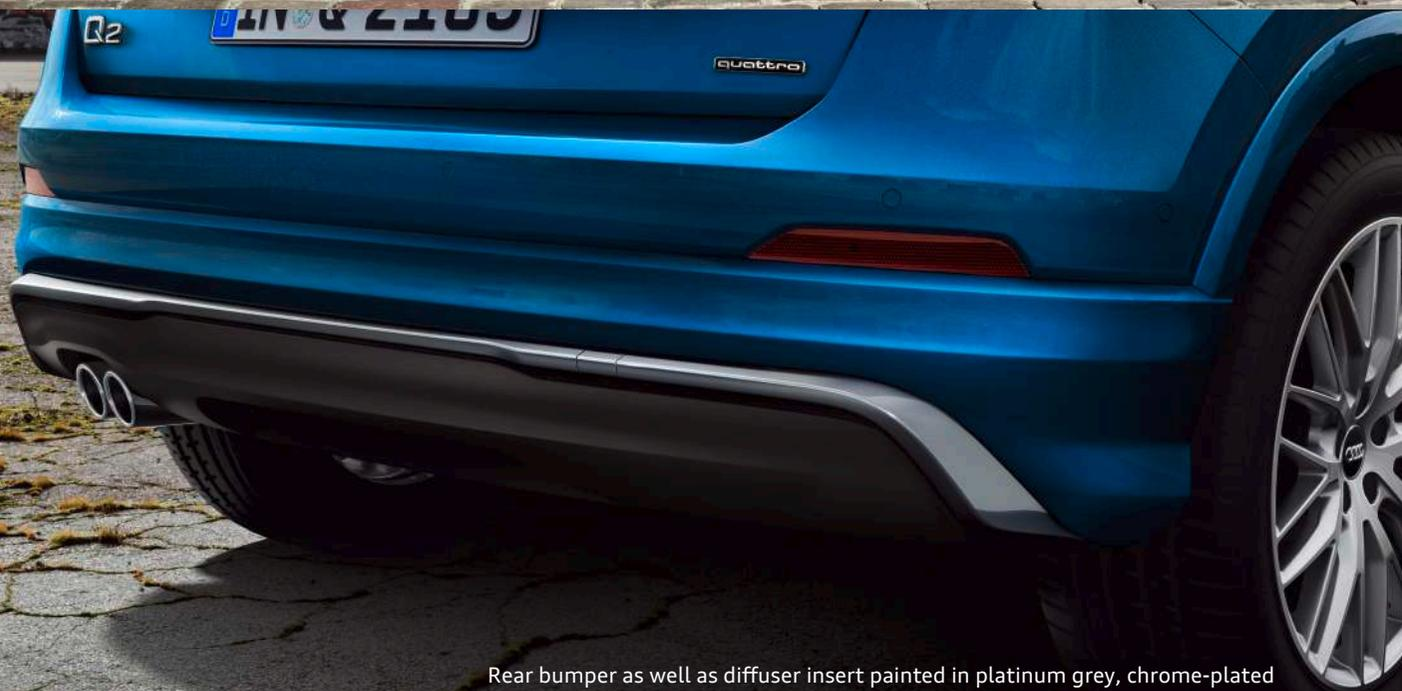
Rear bumper as well as diffuser insert painted in platinum grey, chrome-plated trims for exhaust tailpipes (single or twin depending on engine version)
