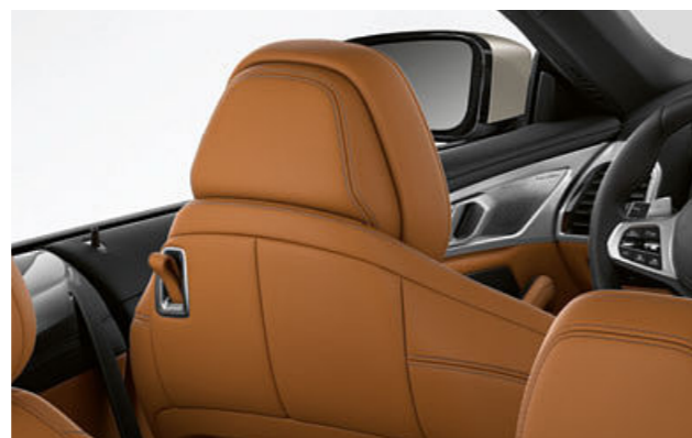
A HIGH-QUALITY GENUINE LEATHER LOOP ON THE BACK OF THE DRIVER AND FRONT PASSENGER SEATS ALLOWS THEM TO BE FOLDED FORWARD QUICKLY AND COMFORTABLY.
