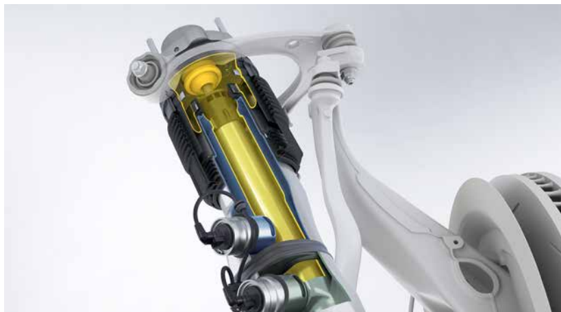
Adaptive air suspension with three-chamber technology
