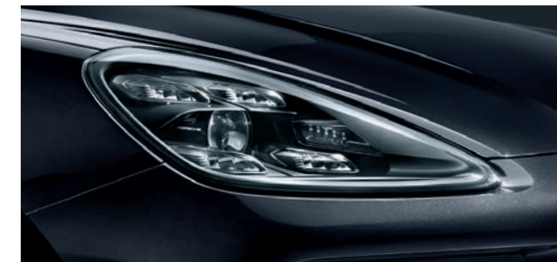
LED main headlights with matrix beam including Porsche Dynamic Light System Plus (PDLS Plus)
