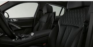
□ The comfort seats for driver and front passenger include active headrests and can be electrically adjusted in various ways. The top part of the backrest, the backrest width, thigh support and headrest height can be individually adjusted. The equipment package also includes the lumbar support and memory function for the driver and front passenger.
