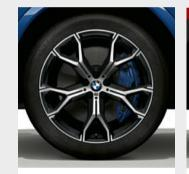
$\Box$  21" M light alloy wheels Y-spoke style 741 M Bicolour Orbit Grey with mixed tyres, gloss-lathed, front 9.5J x 21 with 275/40 R21 tyres, rear 10.5J x 21 with 315/35 R21 tyres.<sup>2,3</sup>
