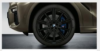
O The high-quality 22" M Performance light alloy wheels Star-spoke style 749 M are weight-optimised with flow forming and designed in Jet Black matt with the M Performance lettering and the colour M logo. TPMS summer complete wheel set, wheel size 9.5J x 22 with tyre size 275/35 R22 104Y XL at the front and 10.5J x 22 with 315/30 R22 107Y XL at the rear.
