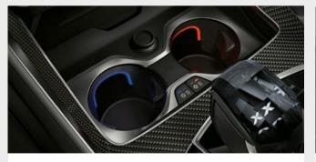
□ The temperature-controlled cupholders in the centre console can individually cool or keep stored beverages warm. The temperature control is activated via buttons on the left and right. The ambient lighting also indicates the function (blue for cooling or red for heating).
