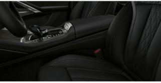
□ In warm weather, the Active seat ventilation, front\* provides a cool and pleasant seat temperature, resulting in a more comfortable driving experience. Air vents in the seat surfaces and backrests suck air. The intensity of the airflow can be adjusted. The perforated surfaces are made of leather 'Vernasca'.
