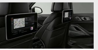
□ Rear-seat entertainment Professional includes two separate high-resolution 10.2" colour screens with touch function that can be tilted and a Bluray drive. In this way, it becomes possible to use navigation and internet functions while driving (if a mobile phone contract exists). Additionally, a USB port and connections for MP3 players, game consoles and headphones (even wireless) are included.
