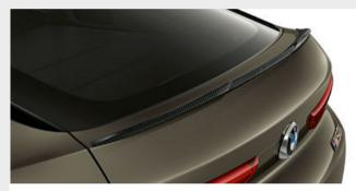
□ The M Carbon\* rear spoiler emphasises the vehicle's powerful, sporty design and noticeably reduces unwanted aerodynamic uplift on the rear axle.
