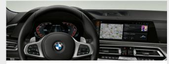
■ The BMW Live Cockpit Professional with navigation function<sup>1</sup> includes two high-quality displays consisting of a high-resolution 12.3" Control Display that can be operated by touch and a fully digital 12.3" instrument display.
