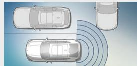
□ The **Crossing traffic warning rear\*** warns you of crossing traffic when pulling out of perpendicular parking spaces.
