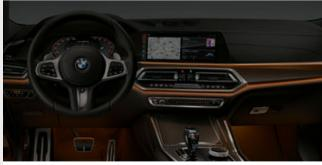
The standard Ambient light, including Ambient contour lighting in the front and rear doors, creates a relaxed, cosy lighting atmosphere in the interior. The Welcome Light Carpet illuminates the area in front of the vehicle doors when entering and exiting. Six dimmable light designs in White, Blue, Orange, Bronze, Lilac and Green are available.
