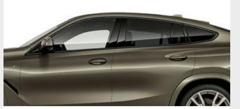
BMW Individual high-gloss Shadow Line<sup>1</sup> includes numerous equipment details in Black high-gloss: the side window frame trim strips, window recess finishers, B- and C-pillars, window guides and mirror bases.
