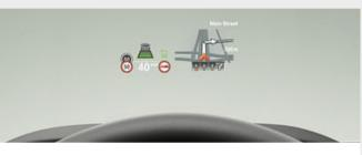
□ The full-colour BMW Head-Up Display<sup>2</sup> projects all information relevant to the journey directly into your field of vision, allowing you to fully concentrate on driving. Information such as the current speed, navigation directions, Speed Limit Info including no-overtaking indicator, along with telephone and entertainment lists are displayed.
