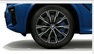
■ 20" M light alloy wheels Star-spoke style 740 M Bicolour Orbit Grey with mixed tyres and runflat tyres, gloss-lathed, front 9J x 20 with 275/45 R20 tyres, rear 10.5J x 20 with 305/40 R20 tyres.
