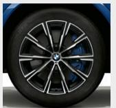
20" M light allov wheels Star-spoke style 740 M Bicolour Orbit Grey with mixed tyres and runflat tyres\*, gloss-lathed, front 9J x 20 with 275/45 R20 tyres, rear 10.5J x 20 with 305/40 R20 tyres.2
