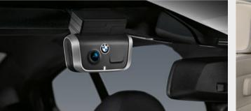
O The BMW Advanced Car Eye 2.0 is a highly sensitive full-HD camera that watches over events in front of and behind the car, even when it is parked. In the event of disturbances and extraordinary movement outside the vehicle, the camera automatically records the situation in order to document possible accidents or (attempted) break-ins.
