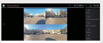
☐ The BMW Drive Recorder\* allows you to record a video from the vehicle environment and play the video on the central Control Display or via USB export also on your CE device. Important vehicle information such as speed and GPS position are stored synchronously with the video. The Drive Recorder has two sub-functions, the Event Recorder and the Crash Recorder.
