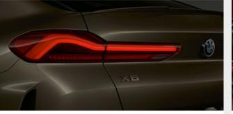
■ The rear lights are made up of individual high-performance LED lighting elements. They have the characteristic, striking BMW L-shape, meaning that the vehicle is clearly recognisable as a BMW even in the dark.
