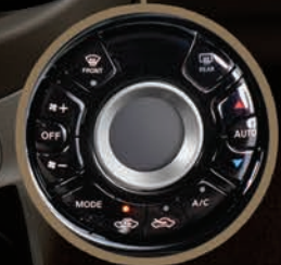
Automatic Air condition
