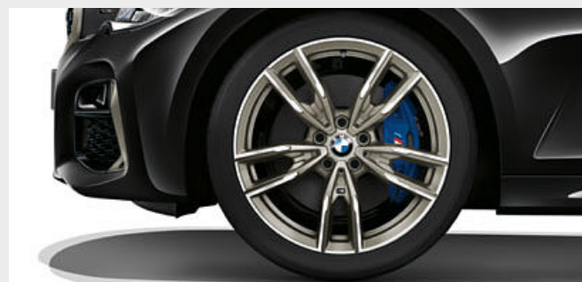
□ 19" M light alloy wheels Double-spoke style 792 M Bicolour Cerium Grey with mixed tyres and runflat tyres, gloss-lathed, front 8J x 19 with 225/40 R19 tyres, rear 8.5J x 19 with 255/35 R19 tyres. 1*
