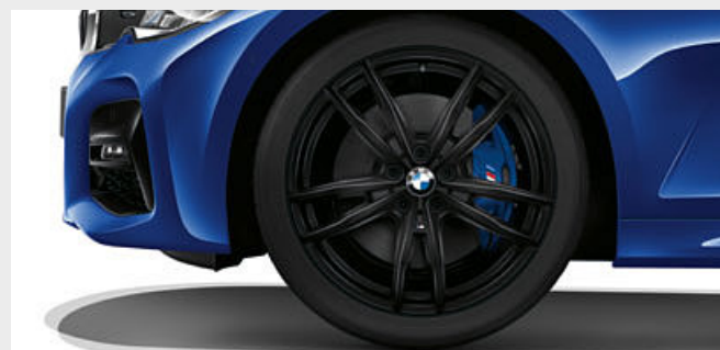
□ 19" M light alloy wheels Double-spoke style 791 M Jet Black uni with mixed tyres and runflat tyres, gloss-lathed, front 8J x 19 with 225/40 R19 tyres, rear 8.5J x 19 with 255/35 R19 tyres. 2
