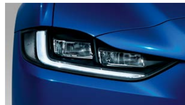
Matrix LED headlights with signature DRL
