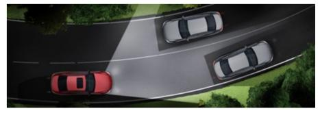
The MULTIBEAM LED headlamps react quickly to the current road and traffic conditions with individually controllable LEDs. The partial main beam masks out other road users detected; when the road ahead is clear, ULTRA RANGE Highbeam switches to permanent long-range illumination of the carriageway.
