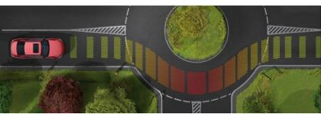
**Route-based speed adaptation** anticipates upcoming road features such as bends, junctions or roundabouts and adjusts the vehicle's speed accordingly.
