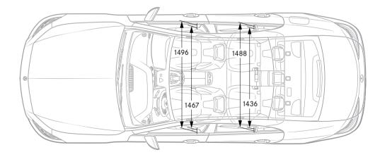
Further technical data may be found at **www.mercedes-benz.com**All figures in millimetres. The dimensions shown are median values. They are applicable for unladen vehicles in the standard specification.
