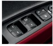
Rear power windows. Unusual in this class, the windows in the rear doors can be raised and lowered at the touch of a button.
