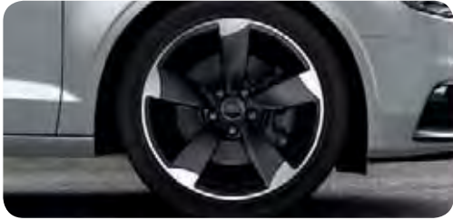
Audi exclusive cast aluminium wheels in 5-arm rotor design in matt black, gloss turned finish size 8 x 18 with 225/40 R 18 tyres 1 . From quattro GmbH
