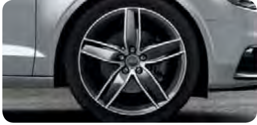
Audi exclusive cast aluminium wheels in 5-arm wing design in glossy titanium look, gloss turned finish 2 size 8 J x 19 with 235/35 R 19 1 tyres 1 . From quattro GmbH
