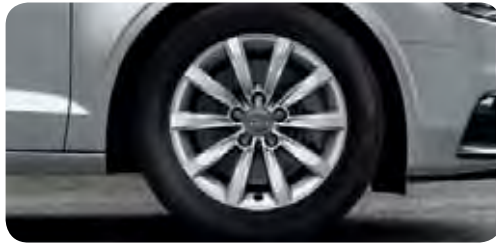
Cast aluminium wheels in 10-spoke design size 7 J x 16 with 205/55 R 16 tyres 1
