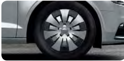
Steel wheels, including full wheel covers size 7 J x 16 with 205/55 R 16 tyres 1
