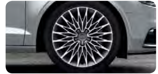
Cast aluminium wheels in multi-spoke design contrasting grey, partly polished, size 8 J x 18 with 225/40 R 18 tyres 1
