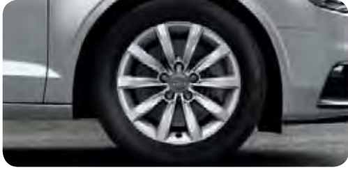
Cast aluminium winter wheels in 10-spoke design size 7 J x 16 with 205/55 R 16 tyres 1 , permissible top speed 210 km/h, cannot be fitted with snow chains
