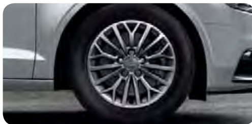
Cast aluminium wheels in 15-spoke Y design size 7 J x 16 with 205/55 R 16 tyres 1
