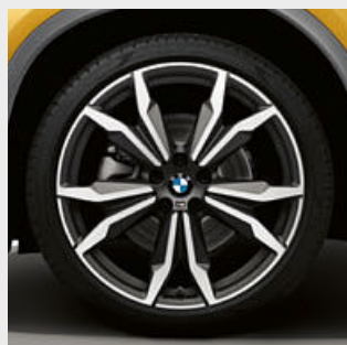
□ 20" M light alloy wheels Double-spoke 2,3,* style 717 M, Orbit Grey matt, gloss-lathed with runflat tyres, wheel size 8J x 20 with 225/40 R20 tyres.
