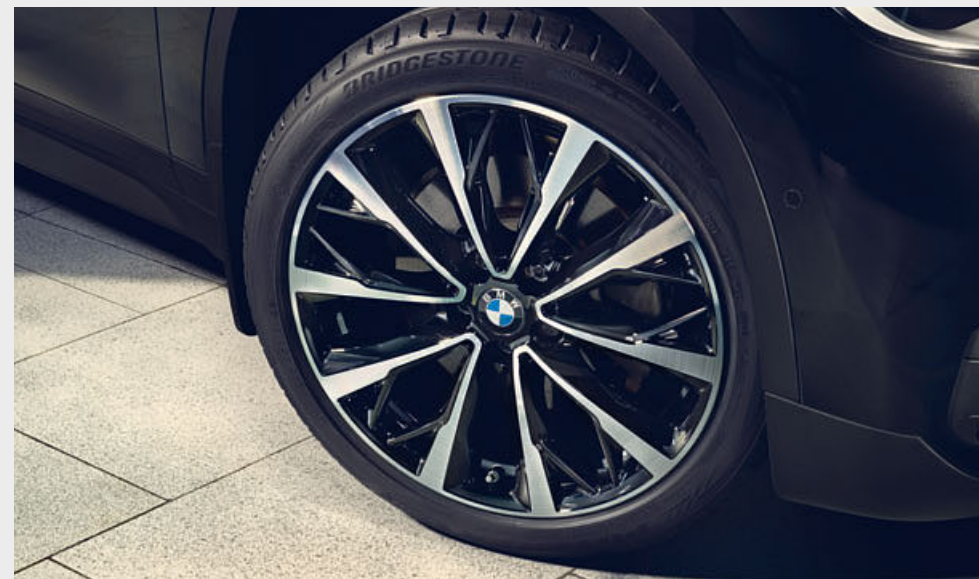
○ The high-quality 19" light alloy wheels V-spoke style 573 are designed in Bicolor Black, bright turned on the visible side and weight-optimised. Summer complete wheel set with run-flat tyres, wheel size 8J x 19 with tyre size 225/45 R19 92W RSC.
