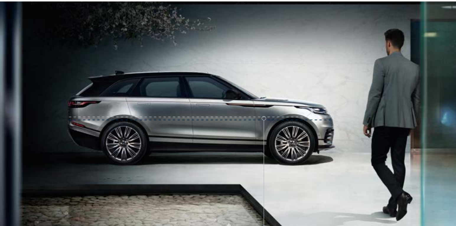
AIR SUSPENSION LOWERS BY 50MM
